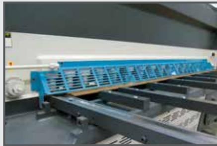
SQUARING ARMS AND FRONT SUPPORT ARMS with or without scale, T-slots and flip over stop. Lengths respectively from 40" up to 120" and from 20" to 120".
